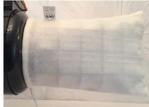
new filter to the frame using the filter ties in the same way you would tie the laces on your shoes. A neat bow!
